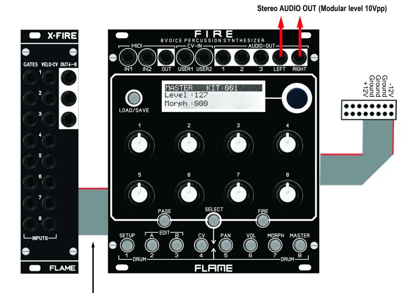
The XFIRE add-on module is connected to the basic module using the approx. 60cm long ribbon cable supplied. This additional module does not require an extra power supply.
