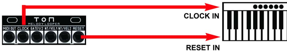
In order for the synchronization to work properly, both devices must be set to the same values for the analog clock and reset. To do this, first go to the SETUP menu of the TON: Press the keys [Fn] > [SETUP] > [#F] one after the other. Use the [TRACK2] key to switch between the two menus Clock out and Reset out:
