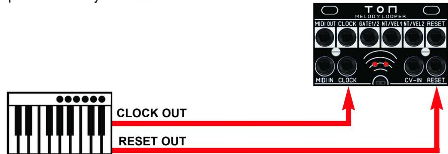
For the synchronization to work properly, both devices must be set to the same values for the analog clock and reset. The TON module has the following non-changeable settings for analog synchronization by an external analog sequencer:
